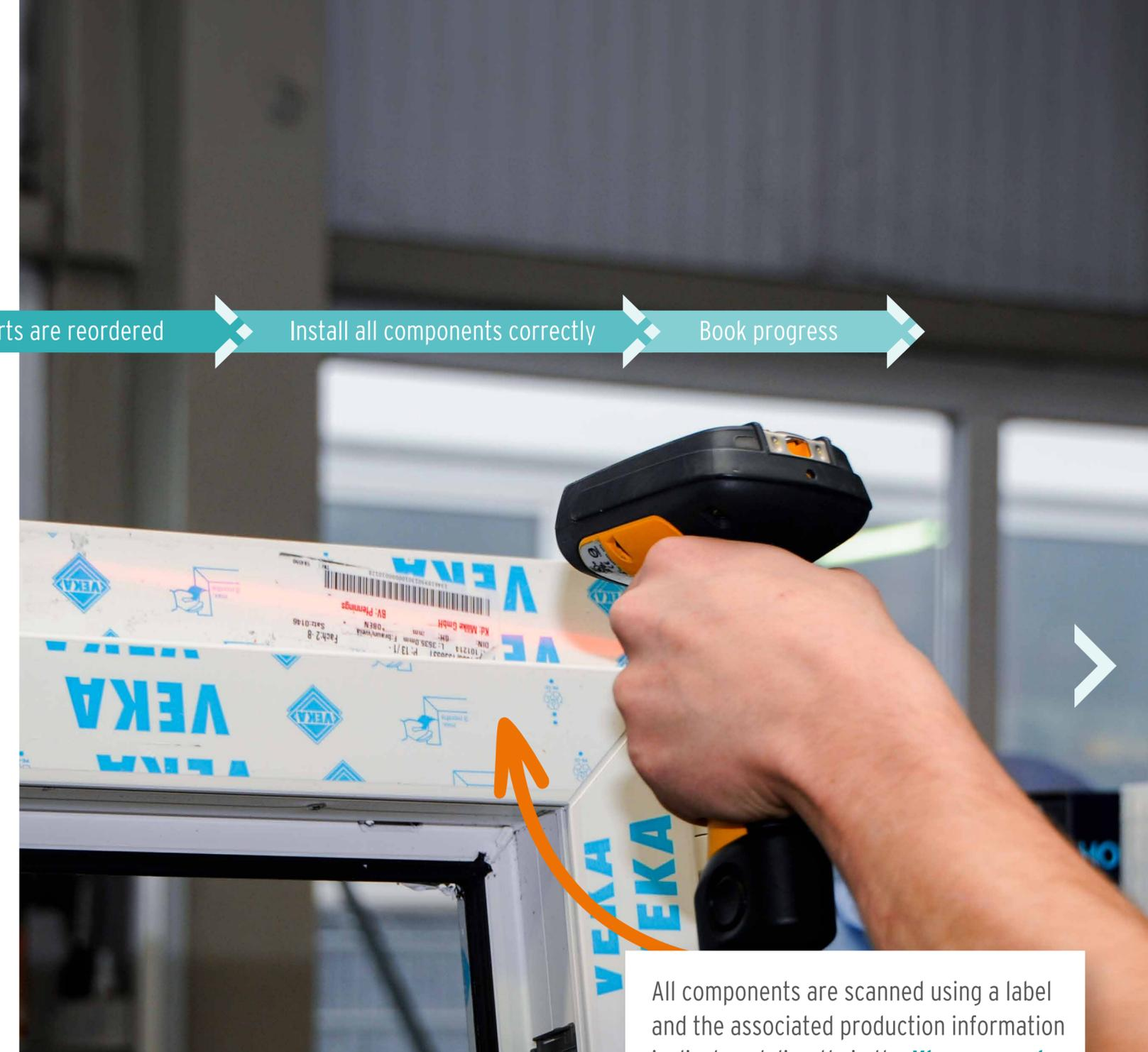
All components are scanned using a label and the associated production information is displayed directly in the **Klaes e-prod**.
