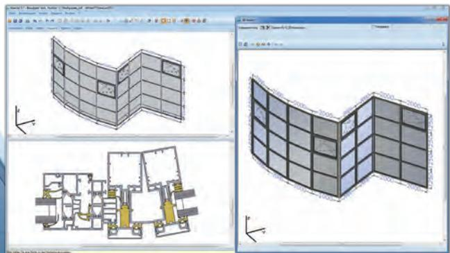
Facade elements are an inherent part of modern architecture. Complex mullion-transom-facades can be constructed in Klaes 3D with ease. Klaes 3D provides you with any production documents and detailed sectional drawings as well as expressive elevations.
