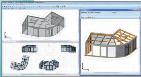
Klaes 3D is based on a highly flexible and open data concept that integrates individual solutions and custom construction methods. You can store your own profile systems and construction details or use existing master data packages and adjust them to your individual requirements.
